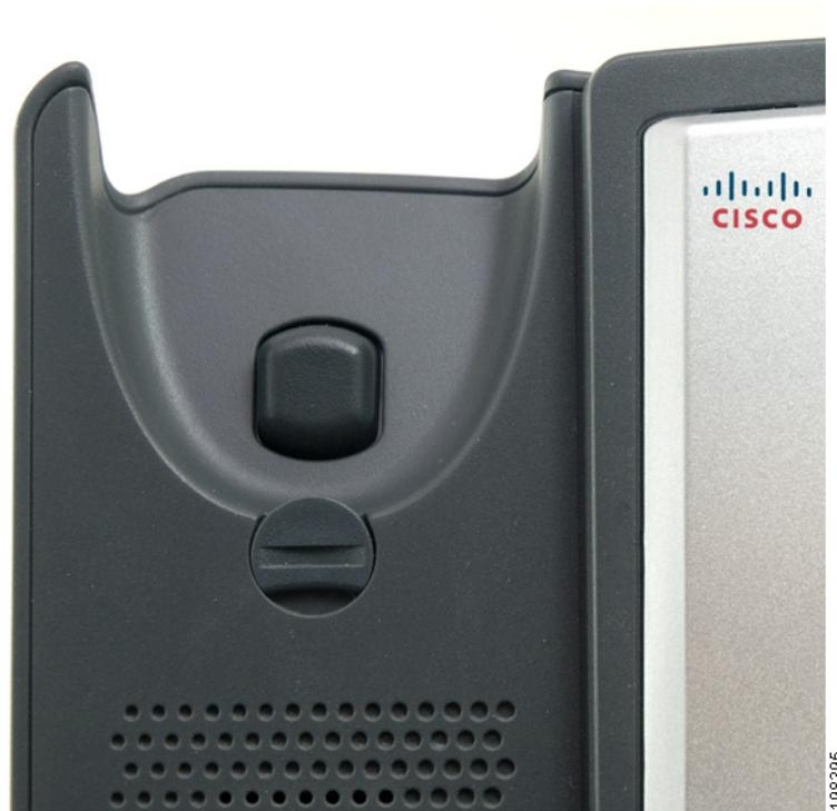
Figure 4 Handset Retention Tab (Reversed)
