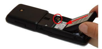
3 Insert battery with the label readable. Align the contacts of the battery with the corresponding connectors on the battery compartment and insert in the direction of the arrow.
