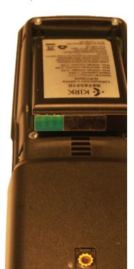
Figure 1-1 Battery Protection Strip
