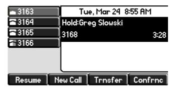
Press  $\binom{\text{Hold}}{}$  again or the **Resume** soft key to retrieve the call. The registered line icon appears as the line indicator.
