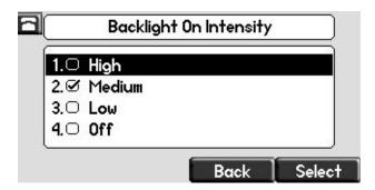
**4.** Use  $\bigcirc$  or  $\bigcirc$  or keypad to select high, medium, low, or off, and then press the **Select** soft key.
