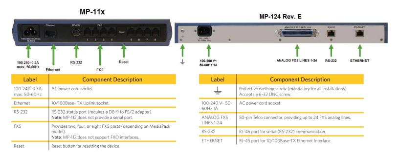
Note: The MP-124 requires an FXS Breakout solution to access the 24 individual phone connection ports.
