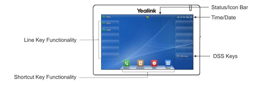
Please Note: DSS Keys provide quick access to the line key screen where the desired line key can be tapped to configure it. There are three types of DSS keys: Line Keys, Programmable Keys, and Ext Keys.
