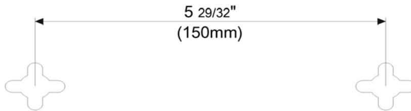
If you install the screws in drywall, use hollow wall anchors to ensure that the unit does not pull away from the wall due to prolonged strain from the cable and power connectors.
