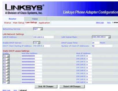
Figure 6-6: Router - LAN Setup Screen
