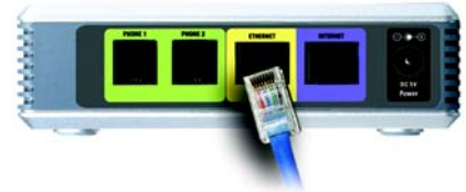
Figure 4-2: Connect a PC
